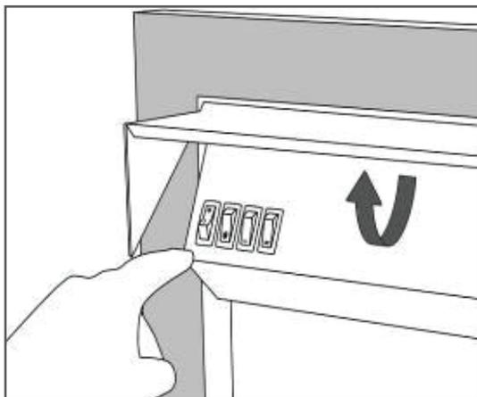
Use the following sequence to operate. The grey represents a 'pressed switch.' A switch is in the ON position when the side with the markings on (e.g. I or II) is 'pressed in'.
