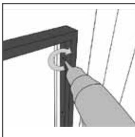
3) Attach the spacer to the surround using 8 x (3.5 x 12mm) screws or similar size
