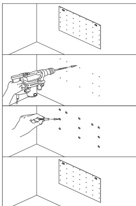
3. Fix the hanger onto the wall and put the fireplace on.
