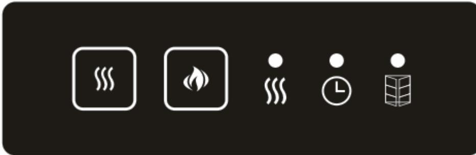
1、 Press key
