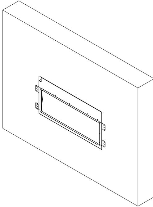
7. Using desired materials, finish to the glass for a clean face installation OR re-attach the steel surround that was removed in STEP 1.
