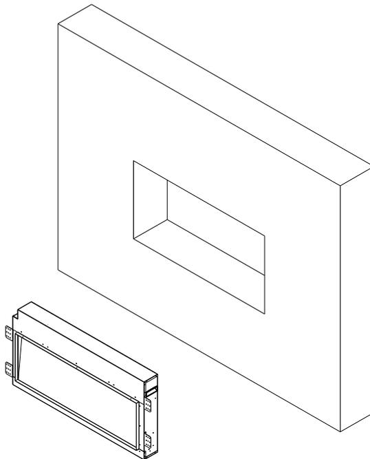
6. Drive the mounting screws through the flaming plates securing the unit into the wall studs.
