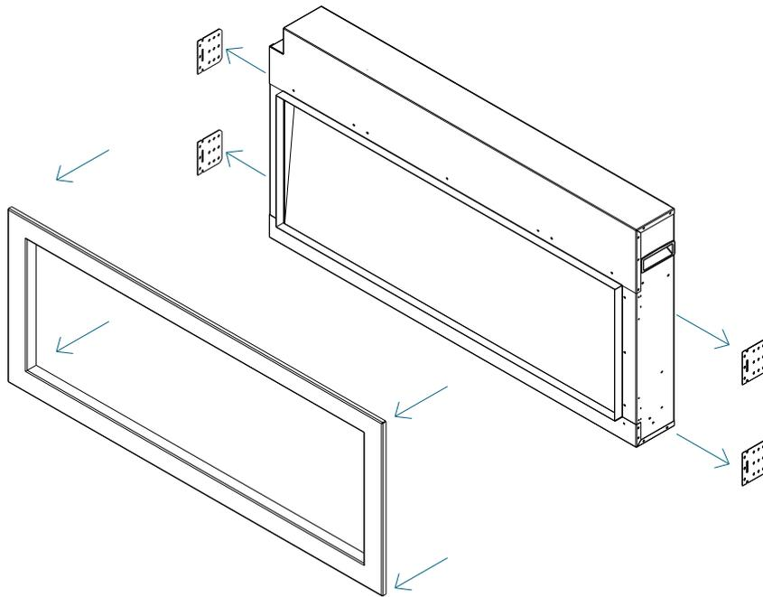
3. Re-attach the framing plates to the unit as shown below.
