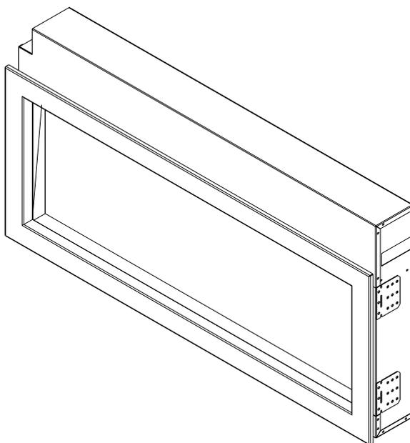
2. Take the hanger from the back of the fireplace by removing screws. Select a location for the hanger to be fixed that is not prone to moisture and is located at least 0.91 m or 3 feet away from combustible materials such as curtains, drapes, furniture, bedding, paper, etc. Before drill, check the wall to ensure there is no wiring, pipe wires etc in the area. Drill 8 or more holes (8mm diameter & 40mm depth) using a suitable size drill and put the wall plugs into the hole.
