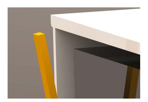
The beams are held in by screws so you will be able to remove them using a screwdriver, then you can push the surround against your wall so it is flush.
