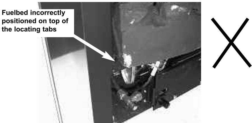
Fig. 16 - Shows incorrect location of fuelbed
