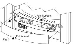
This will then give access to the two lamps. Ensure that the lamps are cool before removing.
