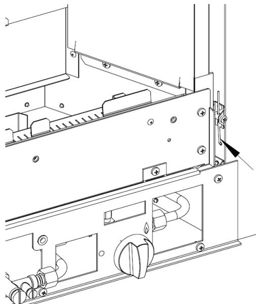
Thread the wire through the small hole below the nipple, then through the nipple as shown. Pull the wire taut to secure the appliance against the back panel. Finally tighten the small screw on the nipple.
