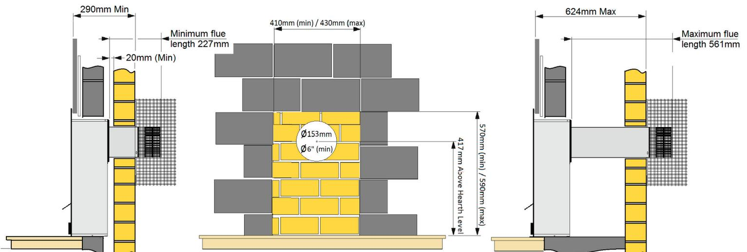
It may be necessary to install a lintel above the cavity that has been created. If a lintel is required to support the recess in the inner leaf (brickwork) then it should either be steel or reinforced precast concrete. The lintel should be the depth of the inner brickwork and be approximately 700mm long.
