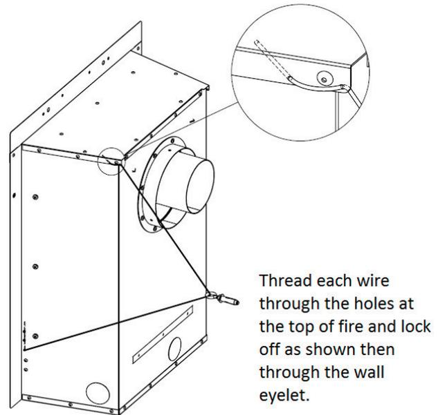
Thread each wire through the holes at the top of fire and lock off as shown then through the wall eyelet.
