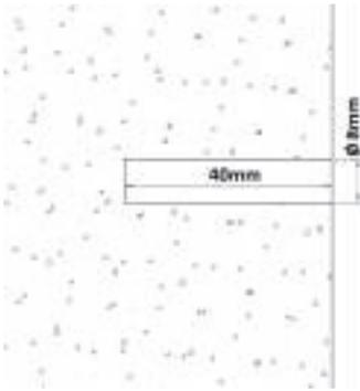
Drill a hole 8mm dia. by 40mm deep. Ensure all the debris is removed from the hole. Use a wrench to twist the nut tightly until the anchor is solid and reliable.
