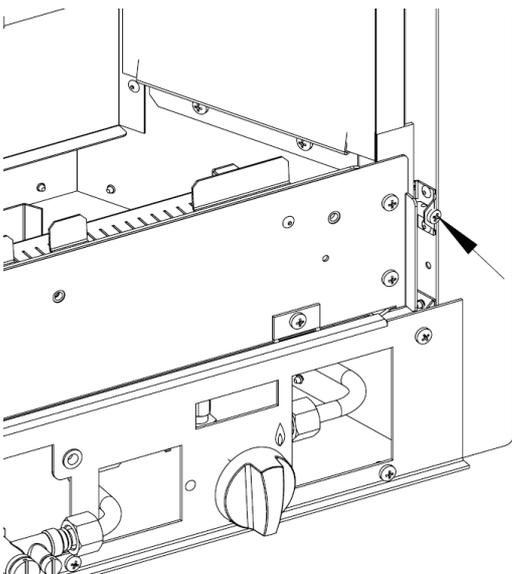
Loosen the nipple screw on each side of the appliance.
